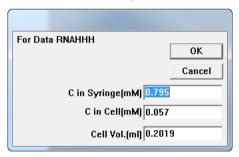
The concentration (*C in Syringe (mM)* and *C in Cell (mM)*) values displayed are those entered by the operator before the experiment starts. Cell volume (*Cell Vol. (ml)*) is constant, which is stored in the data collection software. This value is read by Origin whenever an ITC data file is opened.
