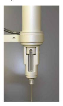
Hold the pipette with an index finger while rotating the syringe with the other hand. When the fill port in the syringe aligns with the opening in the pipette, slide the syringe up approximately another 2 mm.
