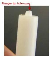
13 Insert the tip pusher and new tip into the pipette and press the tip into place.
