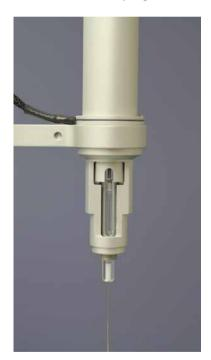
4 Grab the syringe bore firmly and pull straight down to remove the syringe from the pipette. The soft-grip tweezers can be used to help grip the syringe without damaging it. Set the syringe aside.
