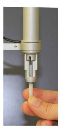
14 In the MicroCal iTC<sub>200</sub> software, click on the *Instrument Controls* tab and click **3.** *New Tip Installed* in the *Maintenance* section.
