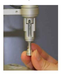
9 In the MicroCal iTC<sub>200</sub> software, click on the *Instrument Controls* tab and click **2.** *Install New Tip* in the *Maintenance* section.
