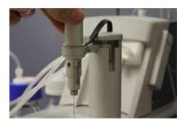
2 Move the pipette and firmly seat into the wash and dry station.
