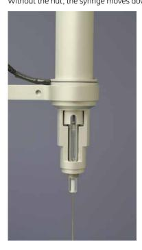
Grab the syringe bore firmly and pull straight down to remove the syringe from the pipette. The soft-grip tweezers can be used to help grip the syringe without damaging it. Set the syringe aside.
