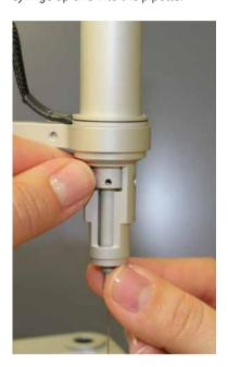
The syringe usually comes to a stop with about 4 mm of syringe glass exposed below the metal. (If it seats directly then there will be about 2 mm of glass exposed and the pipette and syringe can no longer be moved independently.)
