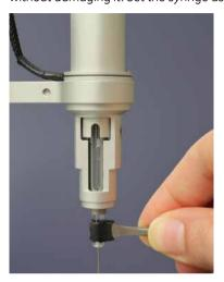
7 The tip of the tip puller uses a traction design that grabs the plunger tip and allows movement only in one direction.
