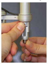
In the MicroCal iTC<sub>200</sub> software, click on the *Instrument Controls* tab and click **1.** *Remove Old Tip* in the *Maintenance* section.
