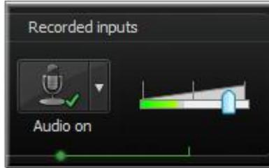
Orange to red warns that you are close to an over-modulated input.
