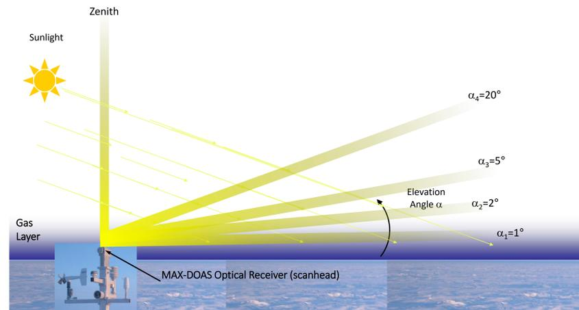
**Figure 1:** Illustration of MAX-DOAS view angles as deployed aboard the OBUOY. Adapted from Hönninger et al., 2004
