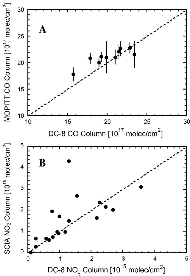
**Figure 7.** Comparison of (a) MOPITT CO and (b) SCIAMACHY NO<sub>2</sub> tropospheric column retrievals with the INTEX-A DC-8 in situ profiles transformed by the corresponding averaging kernels.
