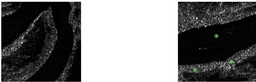
(a) False positive found by the spatial-temporal difference method. This false positive occurred because the GeoJSON does not completely cut out where the land is, and we occasionally get spurious detections on land.
