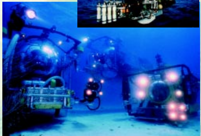
The Johnson-Sea-Link I and II submersibles (left and center) of the Harbor Branch Oceanographic Institution, operate to a depth of 914 meters. Each sub can accommodate one observer and a pilot in the forward acrylic sphere, and a sub crew and observer in the aft observation chamber. The Clelia sub (right) operates to a depth of 300 meters, and carries two observers and a pilot. Each sub can be equipped for a variety of benthic or mid-water sampling applications. Inset: The Johnson-Sea-Link I being deployed with a basket of push corers as scientists prepare to sample cold seep sediments in the Gulf of Mexico.
