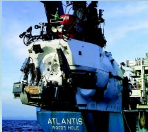
Alvin is a deep-diving submersible that can dive to 4500 meters with one pilot and two observers. It is equipped with two manipulators and sophisticated imaging, attitude sensors and sonar systems and has conducted > 3600 dives during its > 30 year history. It is one of the systems in the National Deep Submergence Facility operated by WHOI for UNOLS.
