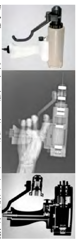
Fig. 2: The prototype of the bone drilling machine (left) as x-ray imaging (middle) and in MRI-imaging in copper sulphate solution (right).
