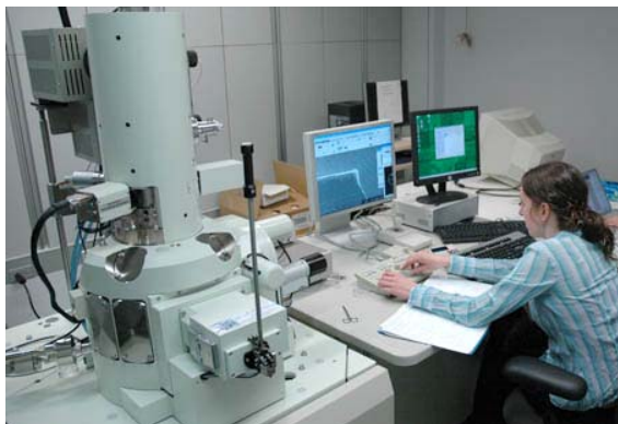
Figure 10.3. Erin Boyd, NSEC graduate student, uses the new JEOL JSM 7000F high-current, e-beam writing instrument in McKay Laboratory.
