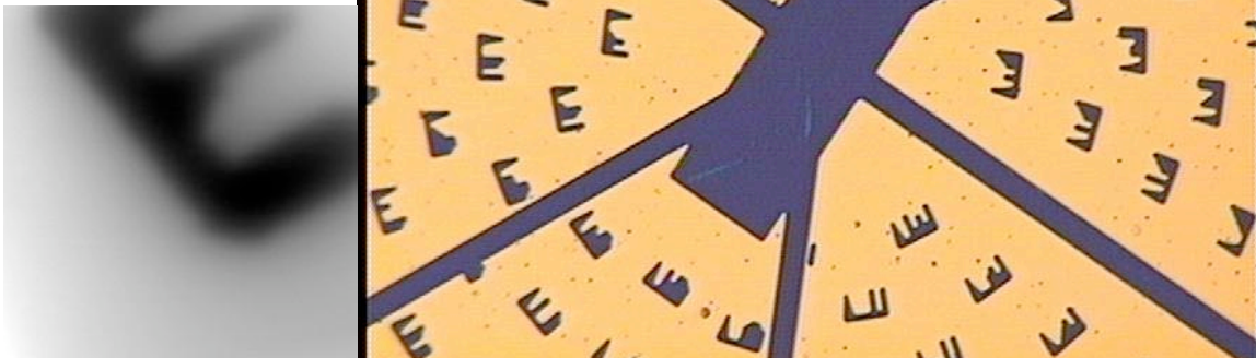
Figure 3.1. ( right ) Pattern of marks for guiding our tip to the location of a graphene piece. ( below ) Image of a mark taken with our capacitance microscope.
