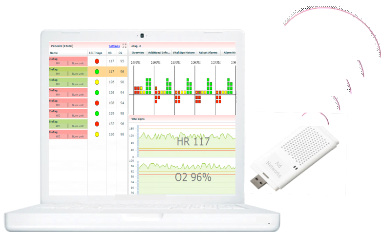
Fig. 3. A USB receiver is used to communicate with the miTags. Patient monitoring software on the laptop sorts patients by triage priority, displays real-time vital sign trends, and processes patient data for alerts.
