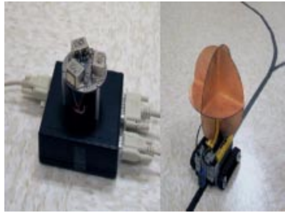
Figure 4: Left: A Doppler radar for tracking moving targets. Right: Target to be tracked.
