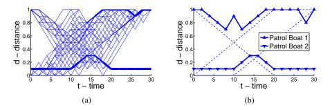
Figure 4.17: Results for sampling under the example setting: (a) Frequency of each edge is chosen when the first sampling method based on Markov strategy is used. (b) Decomposed routes with highest probability superimposed on ferry schedules when the second sampling method based on decomposition is used.
