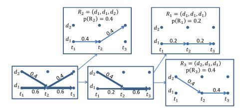
Figure 4.7: Step (i): decomposition. Every time a route containing the minimal flow variable is subtracted and a residual graph is left for further decomposition. The original flow distribution is thus decomposed into three routes  $R_2$ ,  $R_1$ , and  $R_3$  with probability 0.4, 0.2 and 0.4 respectively.
