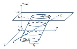
Figure 4.10: An illustration of the calculation of intersection points in the two-dimensional setting. The x and y axes indicates the position in 2-D and the z axis is the time. To simplify the illustration, z axis starts from time  $t_k$ . In this example, there are two intersection points occurring at time points  $t_a$  and  $t_b$ .
