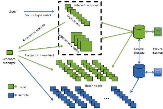
Fig. 2. RCE Hybrid Cloud Architecture. The lower set of batch nodes, storage device, and backup device are “in the cloud”.
