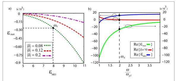
**Figure 2.** (a) Variation of required  $\epsilon_{\text{met}}$  in terms of  $\epsilon_{\text{MO}}$  (for different  $|\delta|$ ) in order to have light-line crossing. (b) Plot of frequency dependence of the relative permittivities of metal and MO medium. The dashed line denotes the parameter values at which the light-line crossing occurs. The values of  $\delta$  are multiplied by 10 in order to be seen more clearly.
