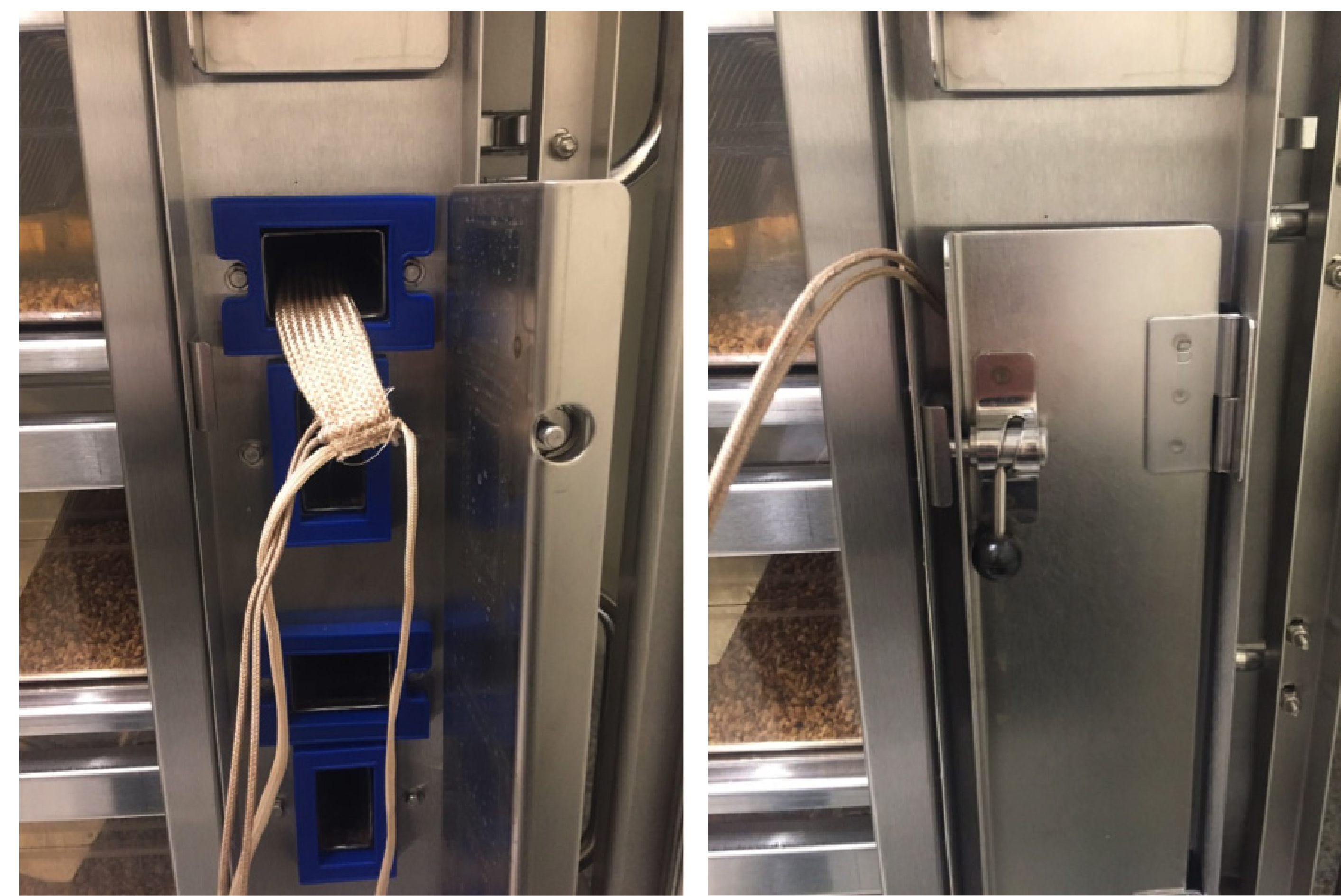
FIGURE 2A AND 2B: HEATING DEVICE INSTALLED IN IVC RACK AIR SUPPLY MANIFOLD
